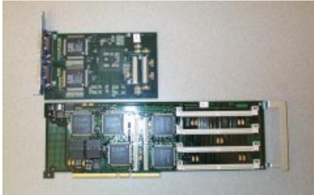
Figure 4: First generation PME prototype with PCI Pamette and Colorado-1 daughtercard. The cards are joined at the PMC connector and face each other in a single PCI slot. Cables attach the daughtercard to the Pixel Bus.
